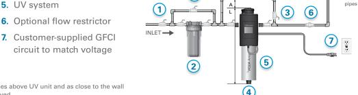
Notes: By-pass pipe should be at least 6 inches above UV unit and as close to the wall as possible to ensure lamp unit can be removed.
