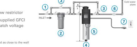
Notes: By-pass pipe should be at least 6 inches above UV unit and as close to the wall as possible to ensure lamp unit can be removed.
