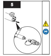
Disconnect the lamp connector from the UV lamp.
