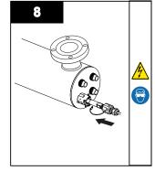
• Connect the lamp connector to the UV lamp.
