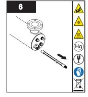
Remove the UV lamp without twisting and discard the lamp.
