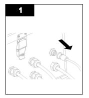
• Disconnect the UV sensor from the controller by disconnecting the sensor cable.
