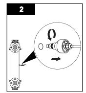
Remove the UV sensor and Oring by grasping the body of the sensor and rotating it counter-clockwise.
