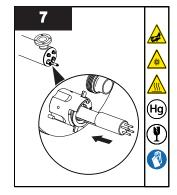
Insert the new lamp fully into the sleeve leaving about two inches of the lamp protruding from the chamber.
