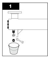
• Remove drain port plug from chamber and drain the water. Replace drain port plug once chamber is drained.
