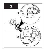
Disconnect the lamp connector and UV lamp from the retaining nut.
