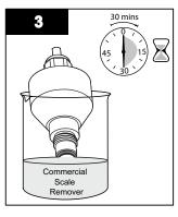
Submerge only the end of the sensor in the commercial scale remover for 30 minutes.
