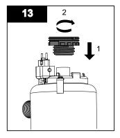
Place new (grey) sleeve bolt onto the quartz sleeve, carefully push down and hand tighten onto chamber.
