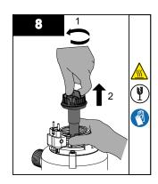
Hold sleeve bolt with one hand and turn lamp counterclockwise and pull the lamp outside the chamber in upward direction.
