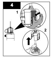
Remove the safety cap by squeezing the tab.
