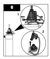
Remove the lamp connector by pulling the tabs out and then upwards.
