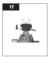
• Connect the sleeve bolt to the top of the sleeve assembly.
