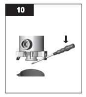
Pry sleeve upwards using sleeve removal tool until it comes loose.
