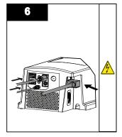
• Plug-in all wires, including power cable.
