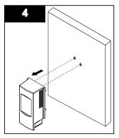
Remove old controller from the wall.
