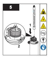
Insert the new lamp fully into the chamber leaving about two inches of the lamp protruding from the chamber.
