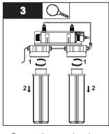
Remove the sump housings using sump wrench.
