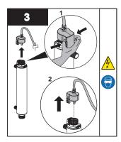
Remove the lamp connector by squeezing the plastic locking tabs on the side of the connector.
