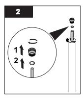
Remove the top retaining nut and O-ring.
