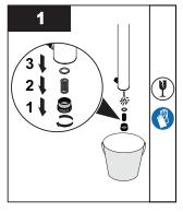
Remove the bottom retaining nut, floating spring, and Oring.
