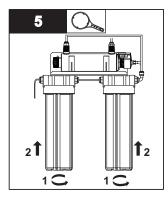
Reinstall the sump housings using sump wrench.
