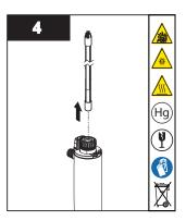
Remove the lamp in upward direction from the chamber and lamp connector base.
