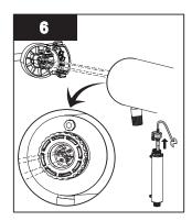
Attach the connector to the UV lamp and note that the connector will only allow correct installation in one position.
