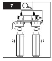
With all faucets closed, remove sump housings using sump wrench.
