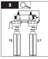
Remove the sump housings using sump wrench.
