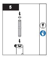
Reinstall the quartz sleeve in the UV chamber allowing the sleeve to protrude at equal distance on both ends of the UV chamber.
