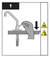
Shut off the water line to UV chamber and release system pressure before servicing.
